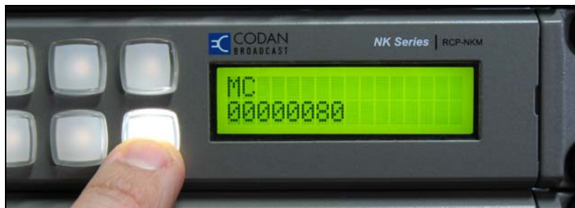
Breakaway Preview Display on an RCP-NKM Control Panel
